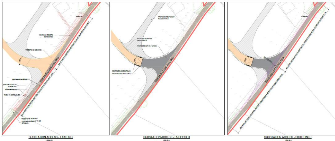
FIGURE 3.3: SUBSTATION ACCESS ASSESSMENT EXTRACT
